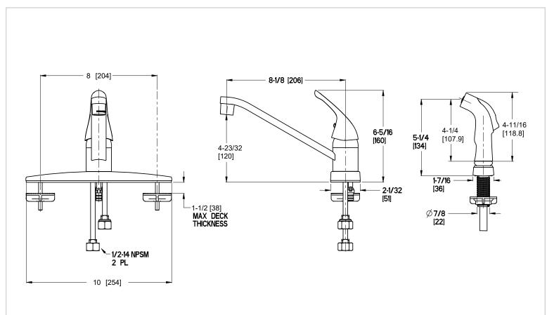
Ø1-3/8 Min to Ø1-1/2 Max. Deck Hole Openings
